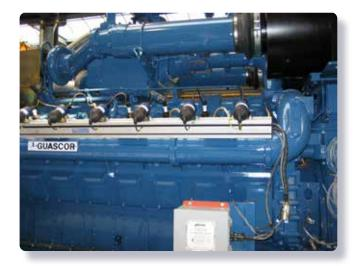
This unique spark plug has been specially designed for the Guascor® HGM560 & Siemens® SGE-56HM. No need to adjust timing or any other settings.
